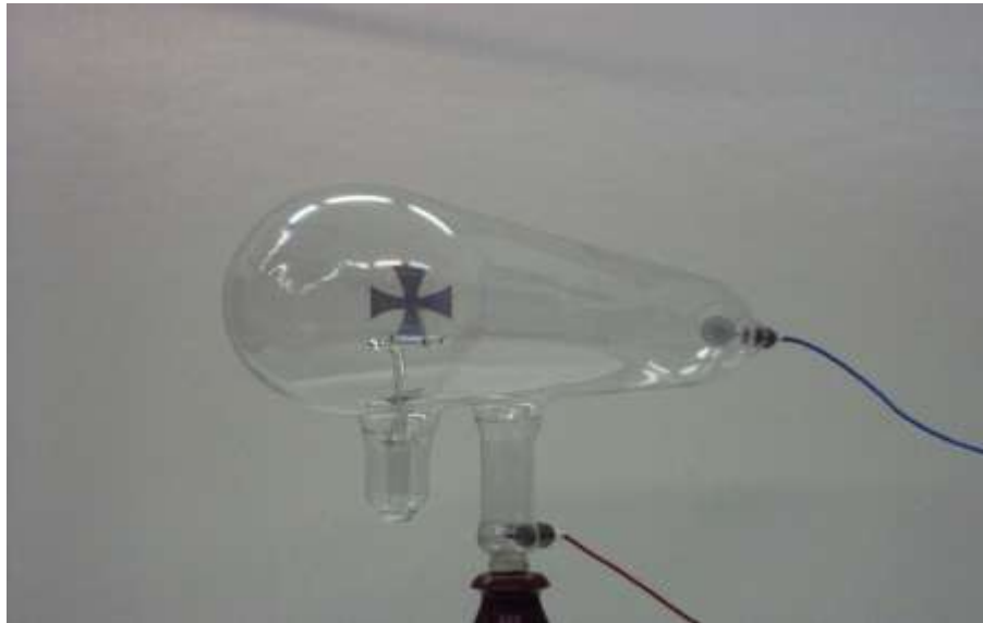
Cathode ray tube. The cathode (negative terminal) is on the right. The anode (positive terminal) is in the base of the tube at bottom.
